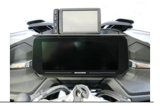
If you are connecting a GPS cradle / mount that is not from BMW, you likely do not have the 3x connector needed to plug into the GPS plug located behind the motorcycle dashboard. Remove fairing speaker to access plug.
